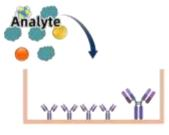
1, Add 100µL standard or sample to the wells. Incubate for 90 min at 37°C. Aspirate and wash plate for 3 times
