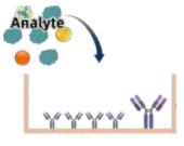
1, Add 100µL standard or sample to the wells. Incubate for 90 min at 37°C. Aspirate and wash plate for 3 times
